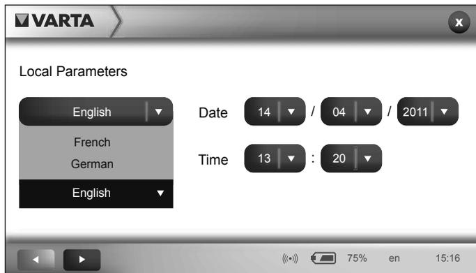
**NOTE** You can scroll through the open list. To do this, tap on the white scroll arrows in the opened list or move stylus upward or downward over the list entries.
